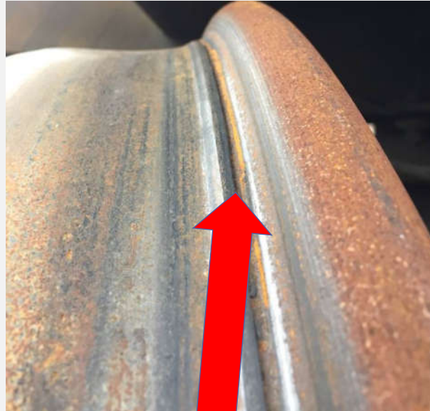
Extraordinary wheel tread deformation near the flange
