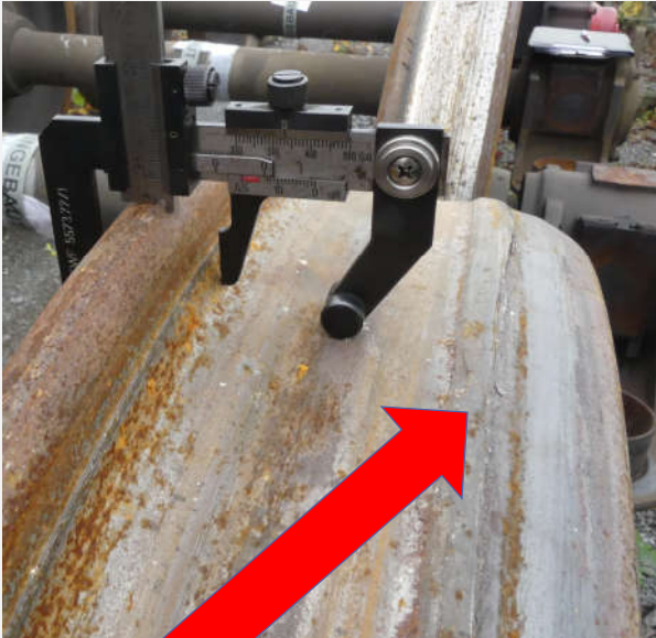
Extraordinary wheel tread deformation on the outer side of the tread
