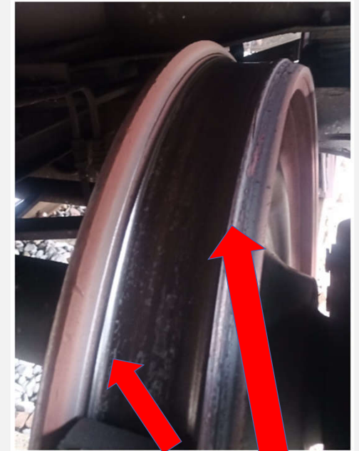
Extraordinary wheel tread deformation on the outer side of the tread and near the flange
